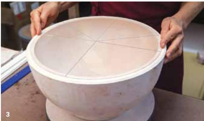
3 Use a circular dividing tool to mark the edge of the mold with guidelines for cutting the slab sections.
