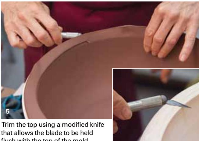
5 Trim the top using a modified knife that allows the blade to be held flush with the top of the mold.
